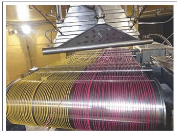
FIG. 1 - Wires being Irradiated
